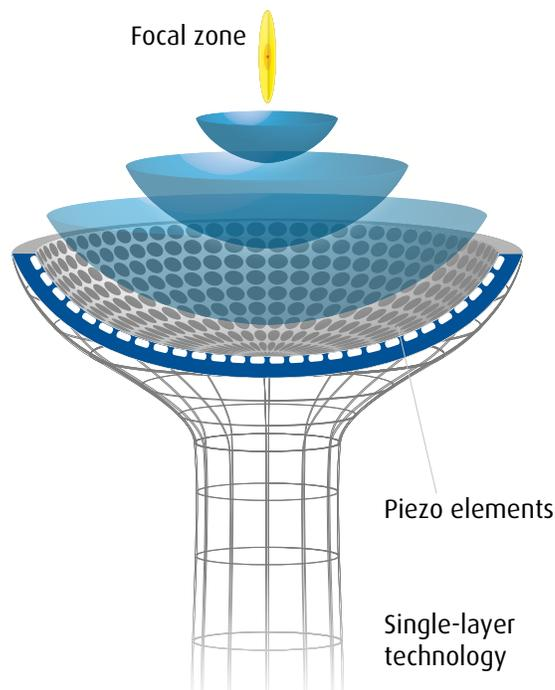
Figure 4 - Piezoelectric shockwave.
