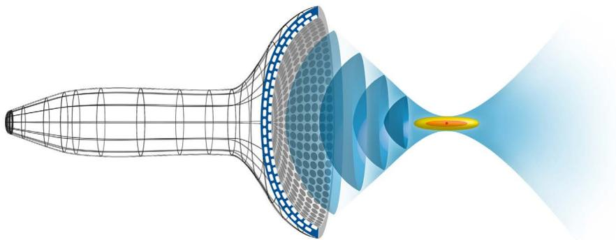
Figure 8 - Example of piezoelectric direct focusing design (no reflectors required).
