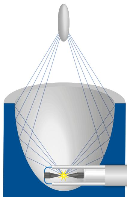
Figure 2 - Electrohydraulic shockwave.
