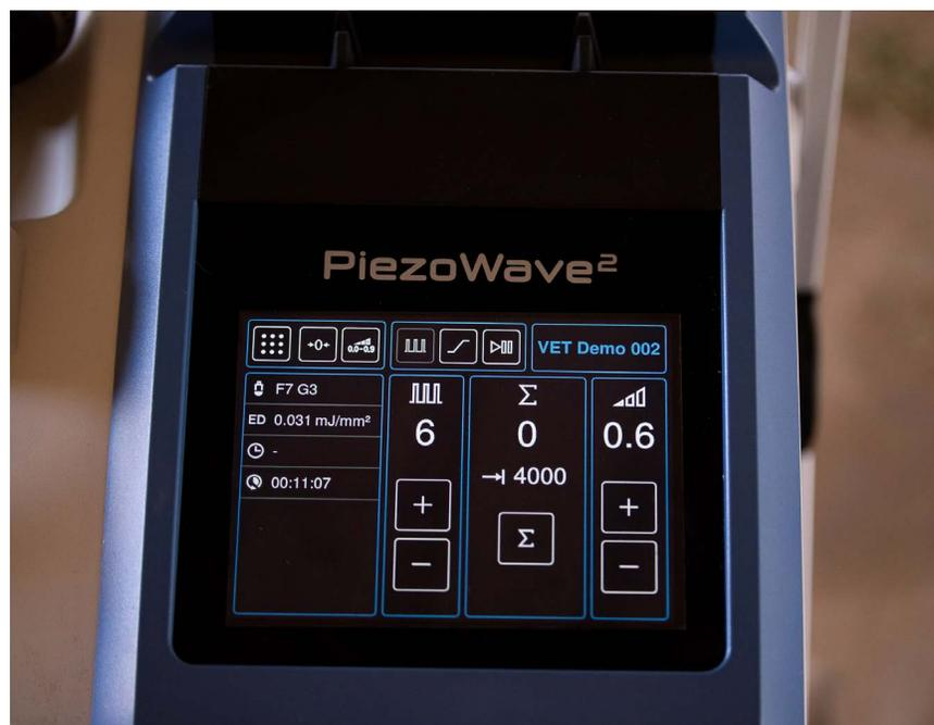
Figure 21 - The left plus and minus keys are used to set the pulse frequency from 0-12.
