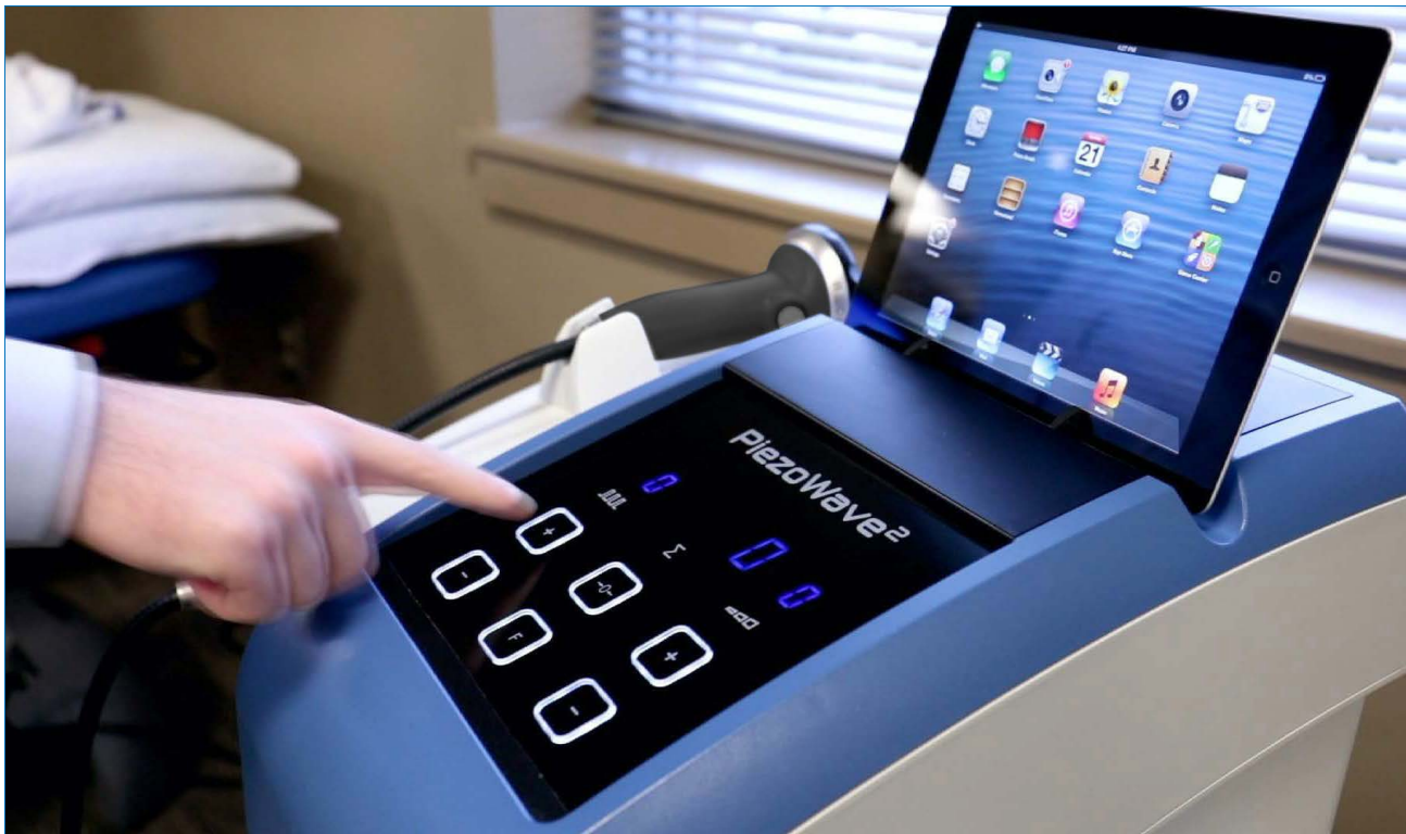
Figure 24 - The left plus and minus keys are used to set the pulse frequency from 0 to 8.
